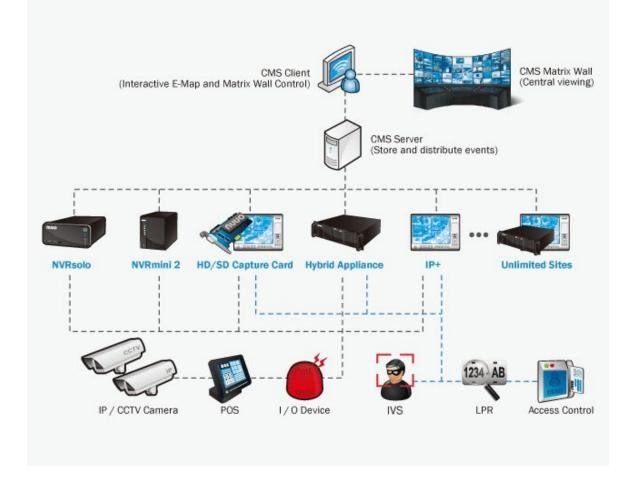
This system have around 100pcs IP camera, we can use 2 sets high performances PC server with NUUO CMS to manage all cameras and NVR in head office, every server manage max 64ch IP cameras. The PC configuration at least is Intel Dual Core i5 / i7 CPU, 4G RAM, 2G Graphic Card, Dual 1000M Ethernet Interface. The video management software on the computer can add, grouping, edit, delete, monitor all cameras and NVRs, user can
